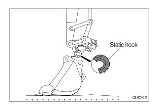
(4) Operate RCV lever to bucket-in position. Then, the moving hook is coupled with the bucket link pin.
