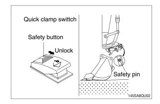
(3) Aligning the arm and bucket, insert static hook of quick clamp to the bucket pin.
